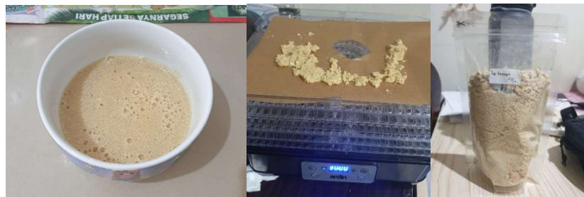
Figure 31. Deposited Corncobs, Corncobs in Dehydrator, Corncobs Starch
