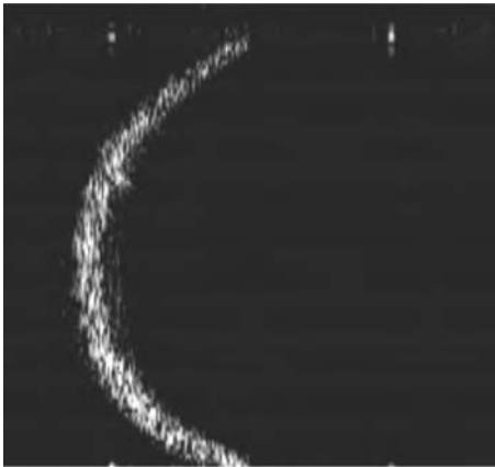
Figure 12.25 Flow velocity profile taken by ultrasonic Doppler velocimetry (UDV).
