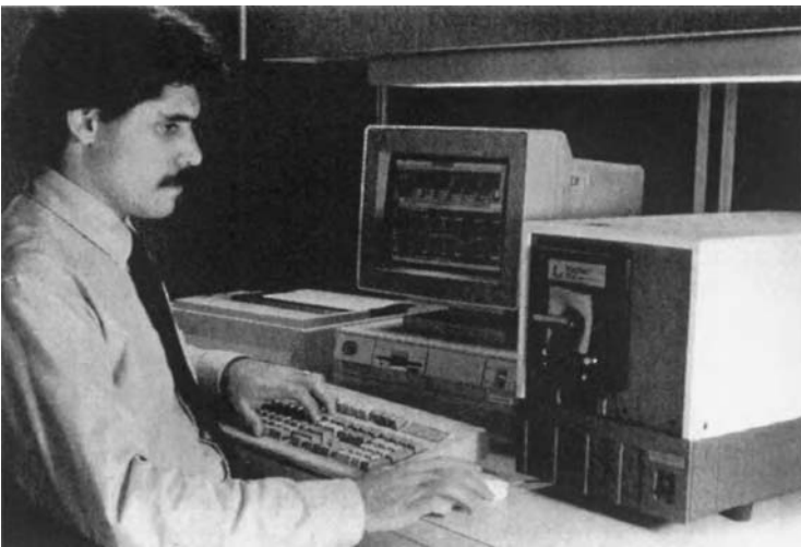
Figure 16.17 The Color-Eye colorimeter. (Courtesy of MacBeth, Kollmorgen Newburgh, N.Y.)
