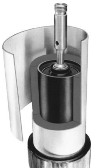
Figure 6.1 Cut-away illustration of fluid in a concentric cylinder rheometer. Courtesy G. Schramm [349]. Copyright 1981, Gebrüder Haake GmbH.
