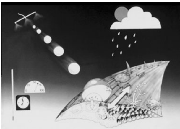
Figure 13.7 Illustration of processes influencing the performance of a crop protection product. Spray droplets impact a leaf surface, and create a foliar deposit from which a pesticidal agent can move into the leaf or contact the fungal or insect pest. From Rodham [865]. Copyright 2000, Elsevier.
