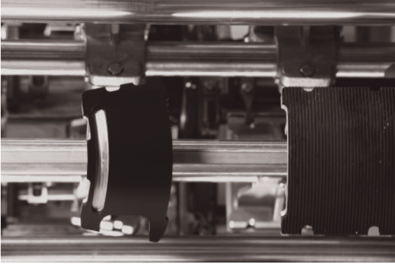
Figure 13.6 The gluing pallets for picking up the foil are designed to be 'glue-free' in the bottle mouth area.
