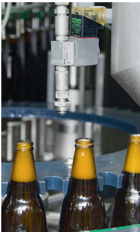
Figure 12.19 Fobber for reducing oxygen in the bottle neck.
